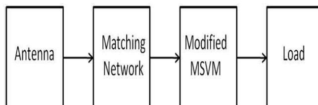
A simple mechanism on how the rectification process works; the antenna gathers or collects the ambient Radio Frequency, then the impedance matching networks boost the collected signals from the antenna to be able to turn on the transistors in the rectifier, then the rectifier converts the collected signal into a DC signal to be fed on the Load. In this work, a conventional voltage multiplier in the rectifier block was modified to achieve a higher voltage output.
